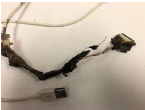
Wire insulation apparently failed, leading to fire.
